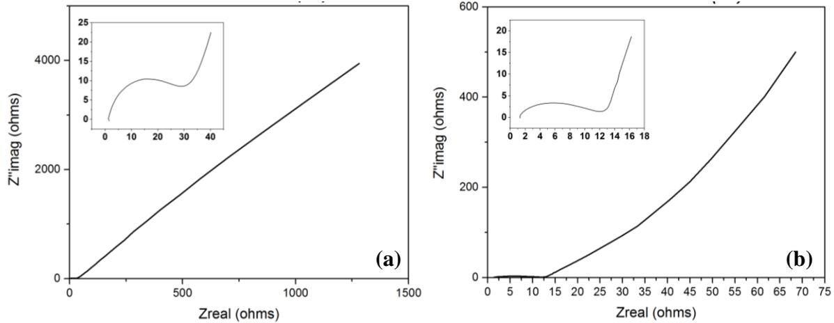
**Figure 4.** EIS (at 1V, in the frequency range of 10 mHz to 300 kHz). The inset to the graphs indicates the high frequency region of the graphs, with a solution resistance ( $R_s$ ) of  $\sim 1 \Omega$  and a charge transfer resistance ( $R_{ct}$ ) of  $\sim 30 \Omega$  and  $\sim 9 \Omega$ , for (a) the basis electrodes and (b) the 500 W plasma processed AC electrodes, respectively.
