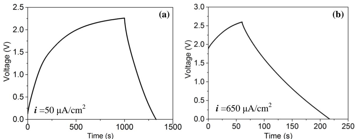
**Figure 3.** Constant current charge/discharge (CCCD) testing was performed on (a) the untreated and (b) plasma treated AC electrodes. The IR drop of the electrodes were  $\sim 385$  m $\Omega$  and  $\sim 460$  m $\Omega$ , respectively.  $V_{max}$  for both curves was set to 2.6 V.
