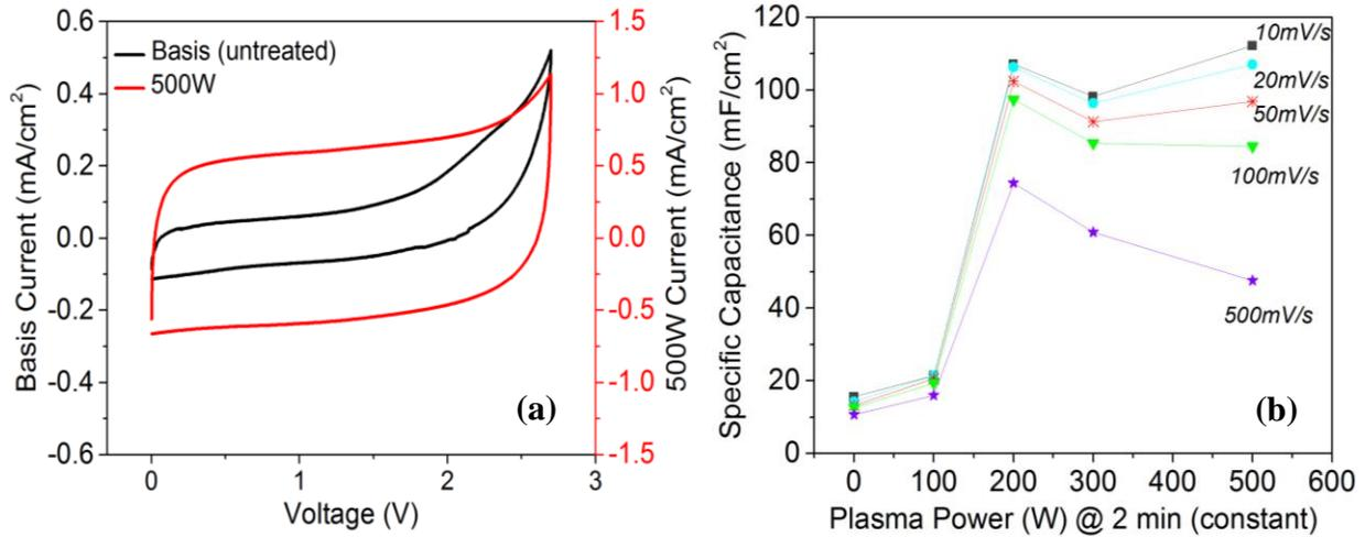
**Figure 2.** Cyclic Voltammetry: AC electrodes were tested at scan rates in the range of 10 mV/s to 500 mV/s, over at least five cycles (averaged values are indicated) in the voltage window of 0 – 2.7 V. (a) the control pair of electrodes (*not* subject to plasma processing) and electrodes, subject to 500 W of argon ion plasma processing at 10 mV/s. (b) Capacitance as a function of Ar<sup>+</sup> plasma power.
