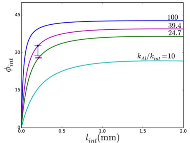
FIG. 4. The heat flux bending angle ( $\phi_{int}$ ) variation with the interfacial thickness ( $l_{int}$ ) as a function of the  $\kappa_{Al}/\kappa_{int}$  ratio, plotted per Eq. (2) and with  $\theta = 45^\circ$ . The marked points correspond to the determined  $\kappa_{Al}/\kappa_{int, alumina}$  ratio of  $\sim 39.4$  and a  $\kappa_{Al}/\kappa_{int, silver}$  ratio of  $\sim 24.7$ .
