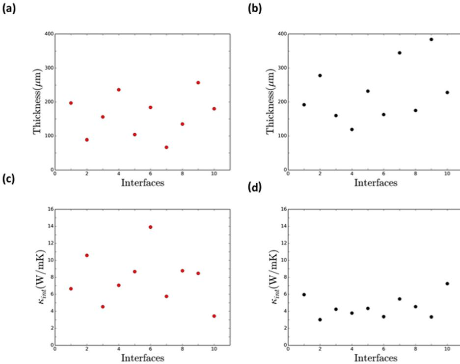
FIG. 3. The measured interfacial thickness variation for the (a) aluminum layer-silver epoxy and (b) aluminum layer-alumina epoxy, joined composites. The estimated thermal conductivity variation for the (c) aluminum layer-silver epoxy, and (d) aluminum layer-alumina epoxy, joined composites.
