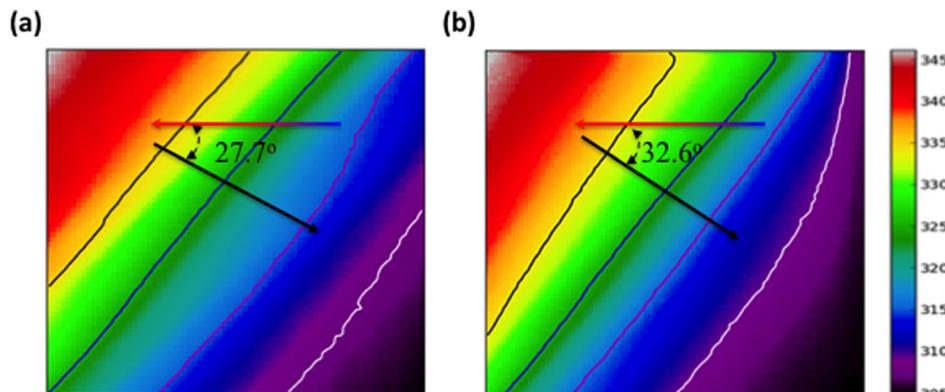
FIG. 2. The steady state transport of heat, as obtained by infra-red imaging, through (a) aluminum layer-silver epoxy and (b) aluminum layer-alumina epoxy, joined composites. The scale bar indicates the temperatures (in K). Typical isothermal contours are at 335 K, 325 K, 315 K, and 308 K, from the left to right. The angles refer to the direction of *net* heat flux bending with respect to a horizontally applied temperature gradient.
