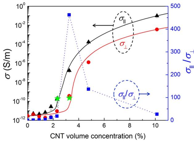
FIG. 2. The variation of the measured electrical conductivity with added CNT filler concentration depicted for the *in plane* ( $\sigma_{||}$ ) and *cross plane* ( $\sigma_{\perp}$ ) configurations. The anisotropy ratio, i.e.,  $\sigma_{||}/\sigma_{\perp}$  is indicated on the right hand axis. The \* indicates the results of the Straley model relating the product of the electrical resistances of the matrix and the filler to the percolation threshold.
