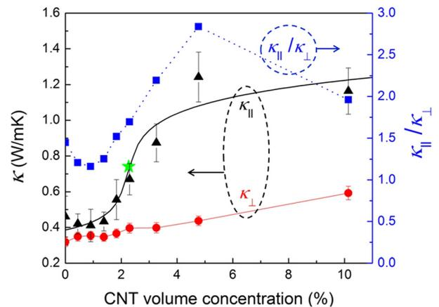
FIG. 3. The variation of the measured thermal conductivity with added CNT filler concentration depicted for the *in plane* ( $\kappa_{||}$ ) and *cross plane* ( $\kappa_{\perp}$ ) configurations. The anisotropy ratio, i.e.,  $\kappa_{||}/\kappa_{\perp}$  is indicated on the right hand axis. The \* indicates the results of the Straley model relating the product of the thermal resistances of the matrix and the filler to the percolation threshold.
