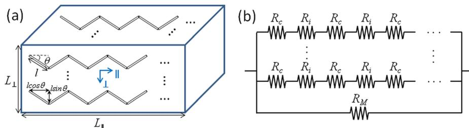
FIG. 4. (a) Modeling networks of aligned MWCNTs in the polymer matrix, and (b) the equivalent electrical/thermal circuit schematic with  $R_c$  as the nanotube resistance and  $R_i$  as the interfacial resistance.
