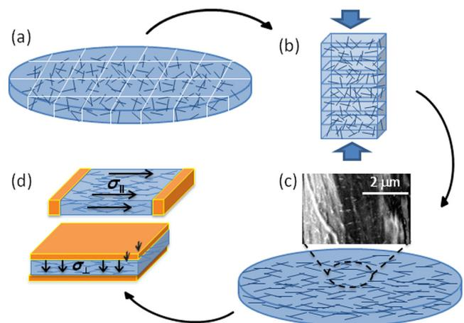
FIG. 1. (a) Blended CNT/polymer composite material was diced and (b) subject to repeated compressive stress. (c) The compressed sheet comprises CNTs preferentially aligned in the plane of the sheet. (d) *In-plane* (top) and *cross-plane* (bottom) electrical and thermal conductivity measurements were carried out to ascertain anisotropy and percolation.
