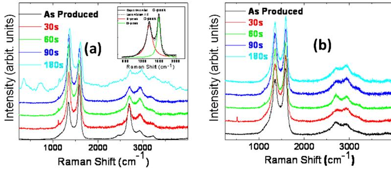
FIG. 2. (Color online) The Raman spectra for the as-produced and Ar exposed (a) BCNTs and (b) HCNTs, irradiated with argon for 30, 60, 90, and 180 s. The inset, in (a) illustrates Lorentzian peak fitting procedures for the D- ( $\sim 1350 \text{ cm}^{-1}$ ) and G-peaks ( $\sim 1580 \text{ cm}^{-1}$ ).
