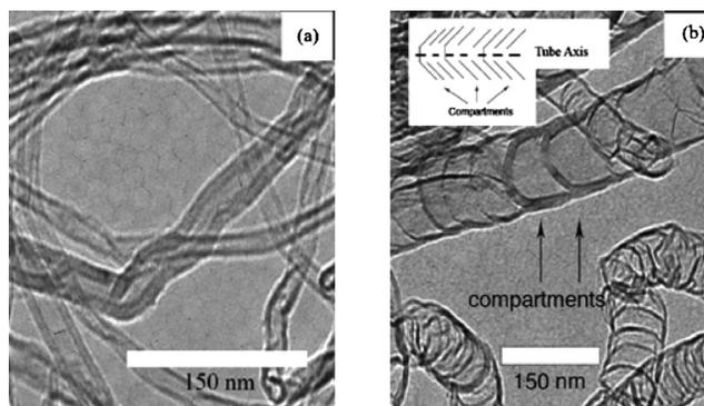
FIG. 1. Transmission electron microscopy images of CNTs of the (a) hollow (HCNT) and (b) bamboo (BCNT) morphology CNTs. The inset of (b) shows the orientation of the graphitic planes.
