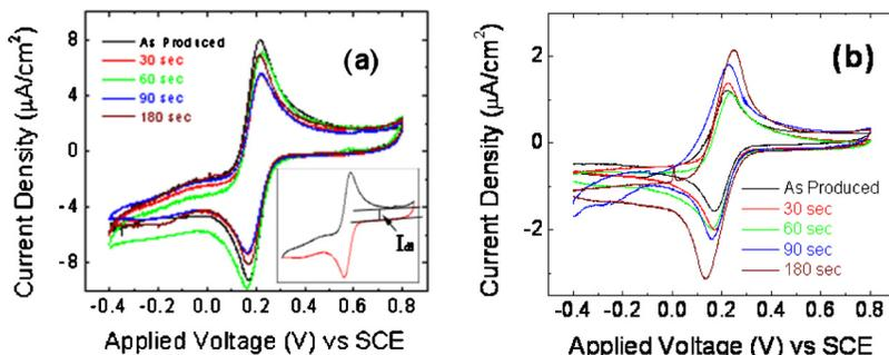
FIG. 4. (Color online) Cyclic voltammograms for (a) BCNTs and (b) HCNTs as a function of increased argon irradiation. The inset in (a) indicates the procedure through which the double-layer current,  $I_{dl}$ , was obtained from a given voltammogram. A scan rate of 20 mV/s with a 3 mM  $K_3Fe(CN)_6$  was used.TABLE V. Characteristics of HCNTs obtained through CV, subject to increasing argon irradiation, where  $v = 20$  mV/s and  $[K_3Fe(CN)_6] = 3$  mM.
