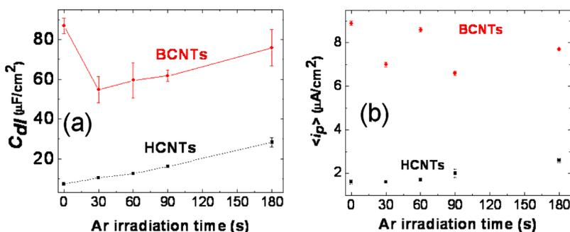
FIG. 5. (Color online) The variation in the (a) double-layer capacitance,  $C_{dl}$  and (b) the averaged peak current density,  $\langle i_p \rangle$ , with argon irradiation time for the HCNTs (black squares) and BCNTs (red diamonds).
