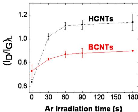
FIG. 3. (Color online) The variation in the line intensity ratio (I<sub>D</sub>/I<sub>G</sub>)<sub>L</sub> for the HCNTs (black squares) and BCNTs (red diamonds), indicates that the former are more amenable to modification.
