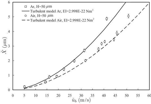
FIG. 4. Experimental (symbols) and predicted (lines) deflections of the CNT tip  $\hat{X}$  in response to hydrodynamic loading by the turbulent flows of argon (squares) and air (circles) for a range of the bulk velocity values  $\hat{u}_b$ . The data from Ref. [5] are for CNTs of height  $\hat{H} = 50 \mu\text{m}$ .
